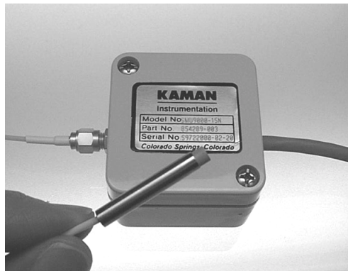
Figure 1. Single Channel SMU-9000.(Poly-carbonate Enclosure shown)
