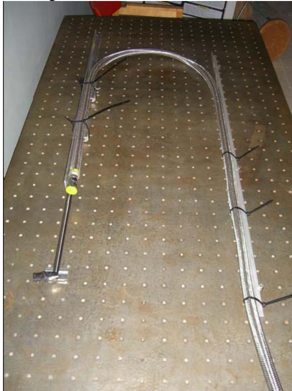
Figure 1: Test set up, right side fixed, left side on linear stage
