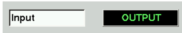
Figure 3: On the left is a control (input) field; on the right is an indicator (read-only) field.
