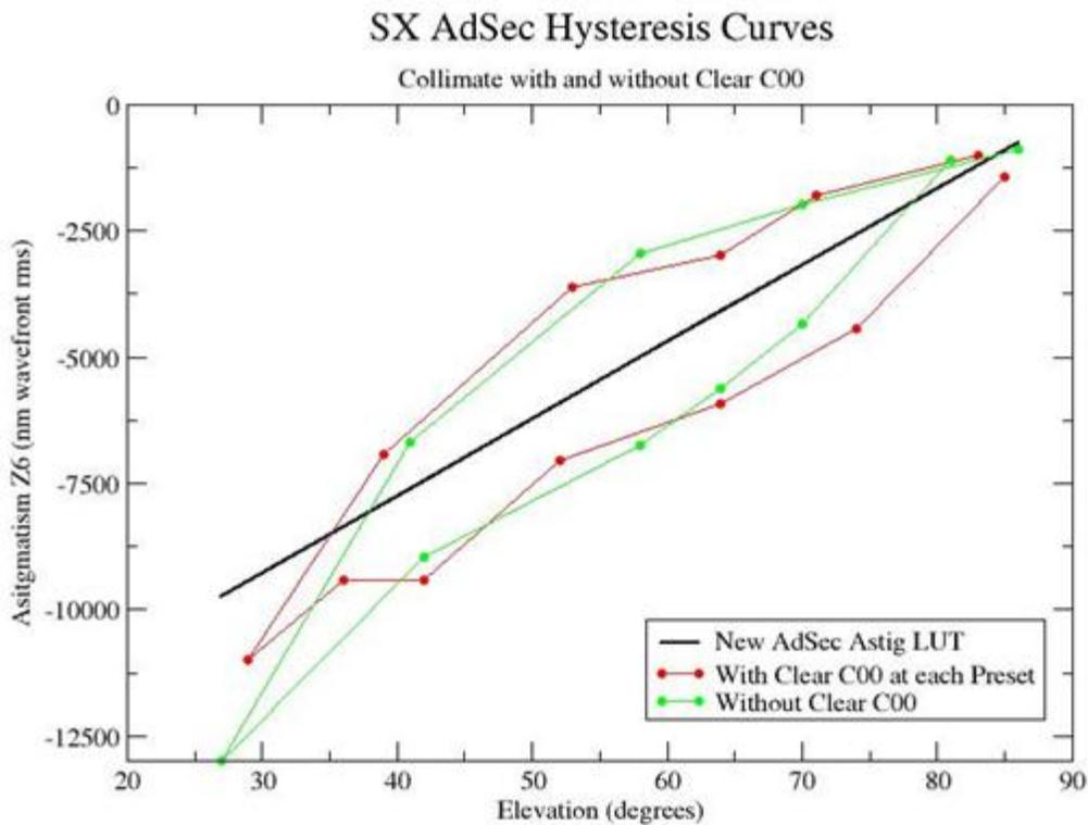
**Figure 5:** Here we show the hysteresis loop for the total astigmatism (Active Optics Z6 + new LUT) vs. elevation. For a set of points, there was a "clear C00" at each preset (red curve), while for the second set, the astigmatism on the primary was the one from the last preset (green curve).
