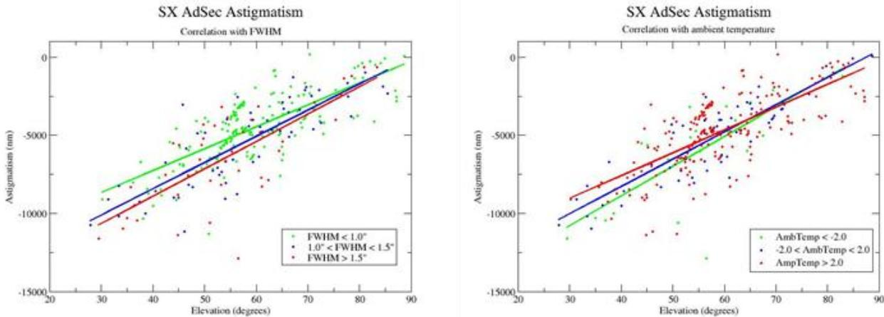
**Figure 3:** Total astigmatism vs. elevation, separated in bins of fwhm (left) and ambient temperature (right). The curves represent the linear fit of the data points in the various bins.
