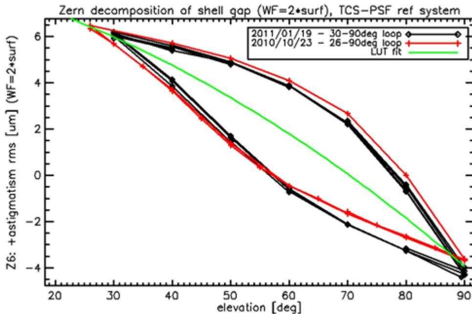
**Figure 1:** Red and black plots represent two samplings of Z6 astigmatism vs. elevation. The green line represents the fitting of the Z6 astigmatism with a 2nd order polynomial to be used for the LUT (plot taken from the FLAO commissioning report [RD1]).
