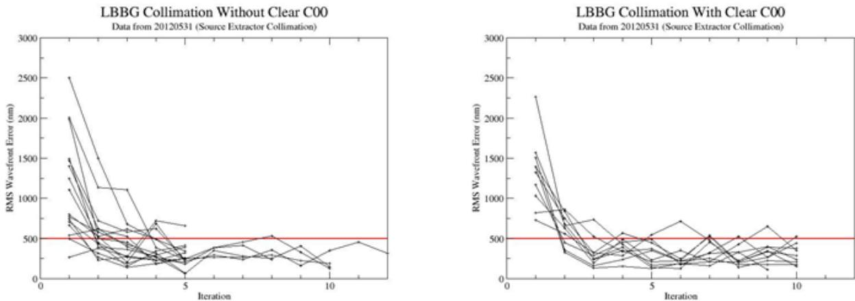
**Figure 6:** Collimation results for the two data sets: without "clear C00" (left) and with "clear C00" at each preset (right).
