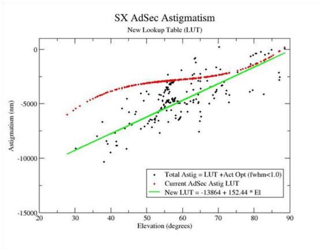
**Figure 4:** The black points represent the total astigmatism vs. elevation for all points obtained with good seeing conditions (fwhm<1.0"). The green curve is the linear fit to these points and will be used as the new LUT. The red points show the original LUT.
