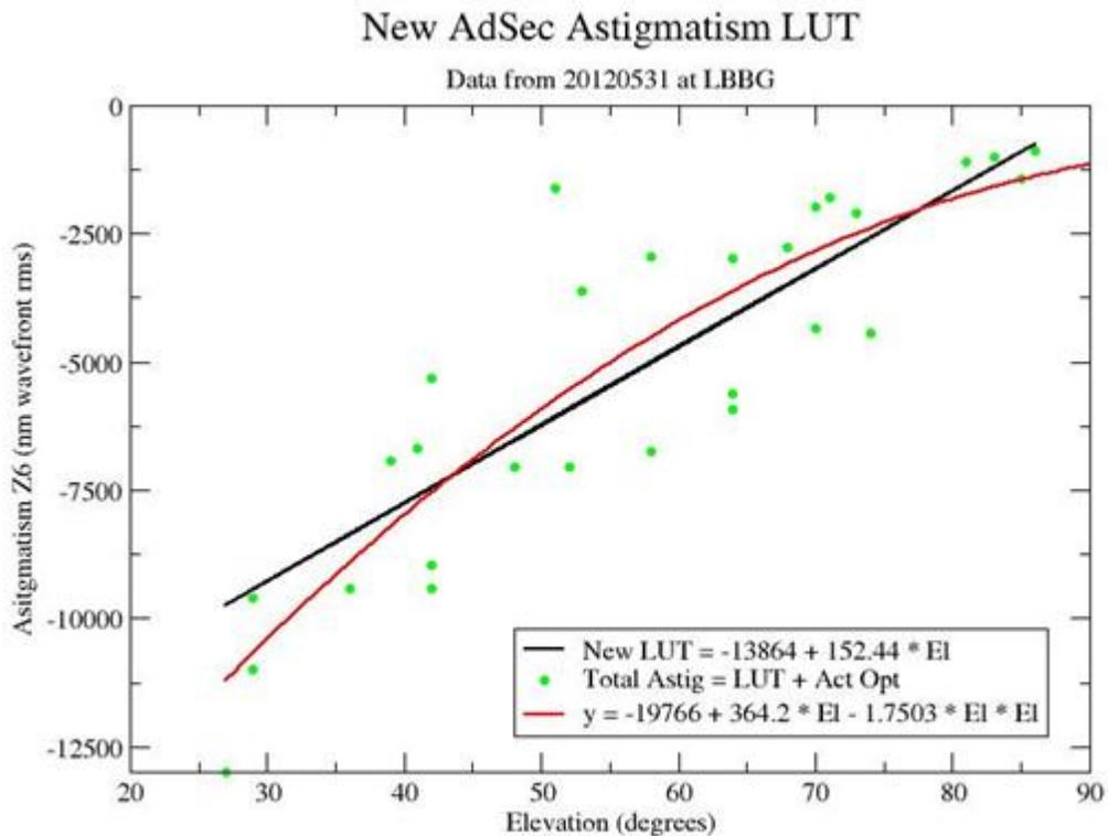
**Figure 7:** Total astigmatism vs. elevation for the data set obtained during the technical run for the verification of the new LUT. Green points represent the measured values of the total astigmatism (new LUT + Z6 from Active Optics). The black line is the linear fit that represents the new LUT and the red curve is a first quadratic fit of these same data, which could represent a future improved LUT.
