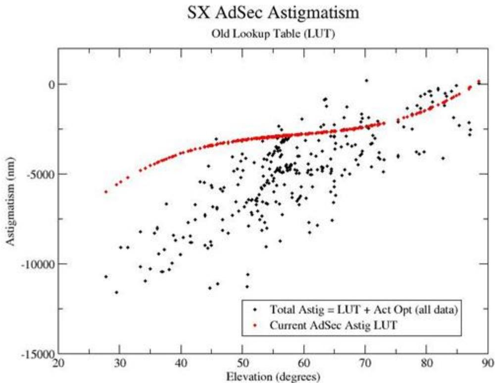
**Figure 2:** Astigmatism vs. elevation for the left adaptive secondary mirror (SX AdSec). Red points represent the original LUT values. Black points represent the total astigmatism that had to be applied to the AdSec for collimation. This total astigmatism is actually the sum of the LUT value and the additional Z6 correction applied by the Active Optics.
