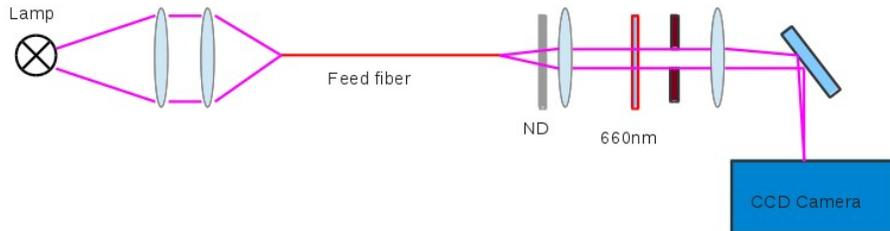
Figure 2: The reference test setup. Here the ARGOS TT system has been replaced by a CCD camera to provide a efficiency reference measurement.
