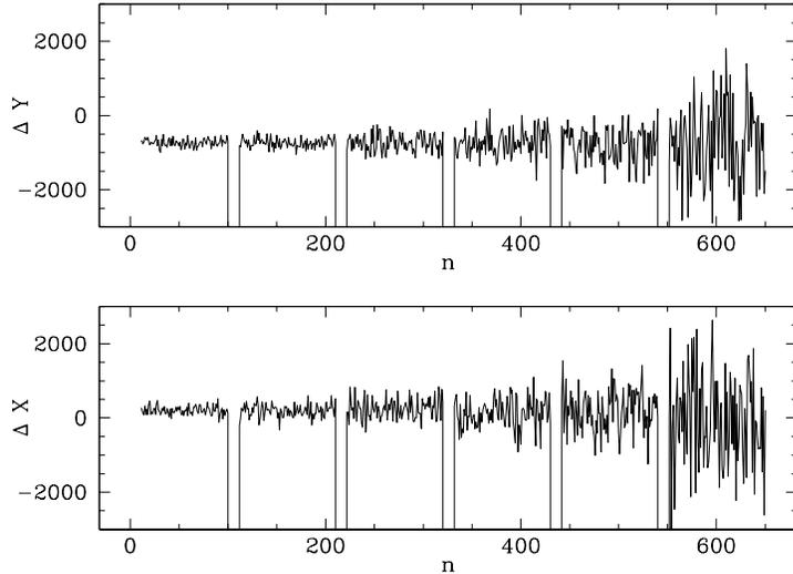
Figure 13: The guide signal in counts in X and Y as a function of sample number (n) for different integration times. From left to right the integration times are 1000, 500, 200, 100, 50, and 10ms.
