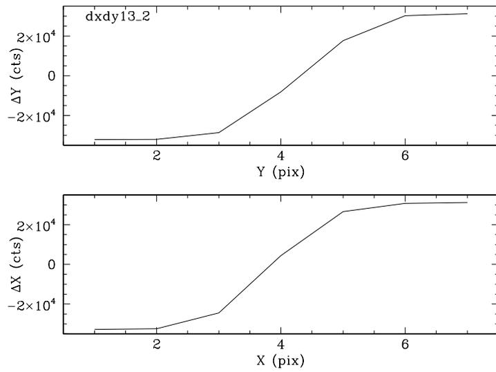
Figure 12: The guide signal in counts as a function of the X and Y position, based on row 4 in the upper left image (dx13\_2; X-offset) of the previous figure and based on column 4 in the upper right (dy13\_2; Y-offset) of the previous figure.
