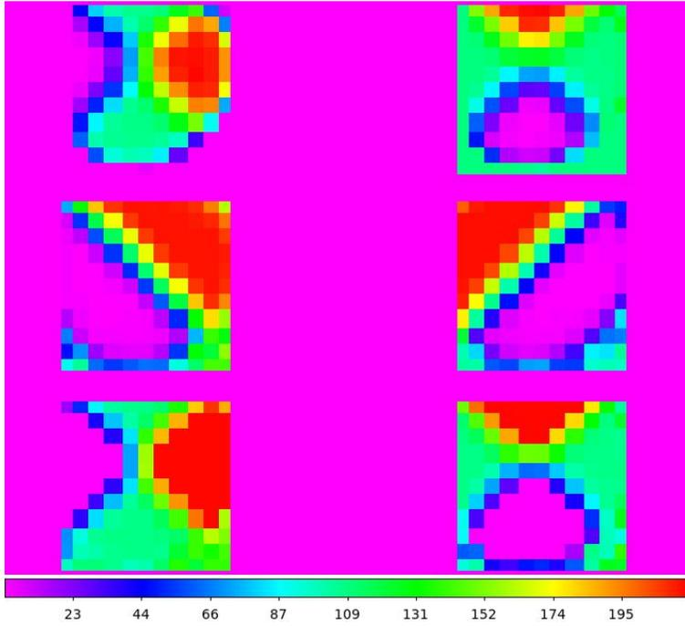
Figure 9: The guide signal as a function of raster position. The middle row of images show the offsets in X (left) and in Y (right) as a function of raster position. The upper row shows the offsets in X (left) and Y (right) after the rotation of 45 degrees has been taken out by the TT computer. The lower row is the same as the upper row except that the computations have been done directly from the images in the middle row.
