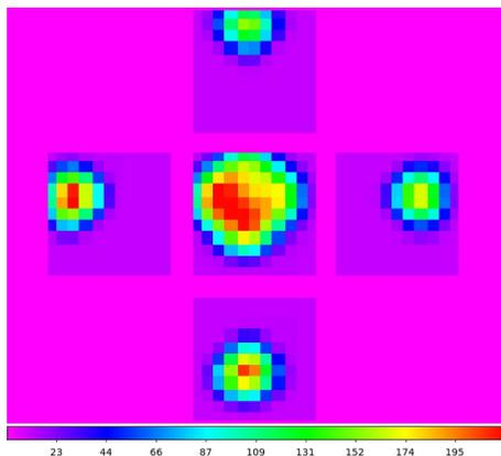
Figure 3: The signal as a function of  $(x,y)$  position in a raster scan with step size  $500\mu\text{m}$ . The outer four images represent the response of the individual channels while the center image is the sum of the four outer images and thus representing the overall sensitivity of the array. In this case the channels have been dark subtracted and corrected for the APD flatfield leaving the relative sensitivities. The intensity scale ranges from  $-0.05$  to  $1.0$ .
