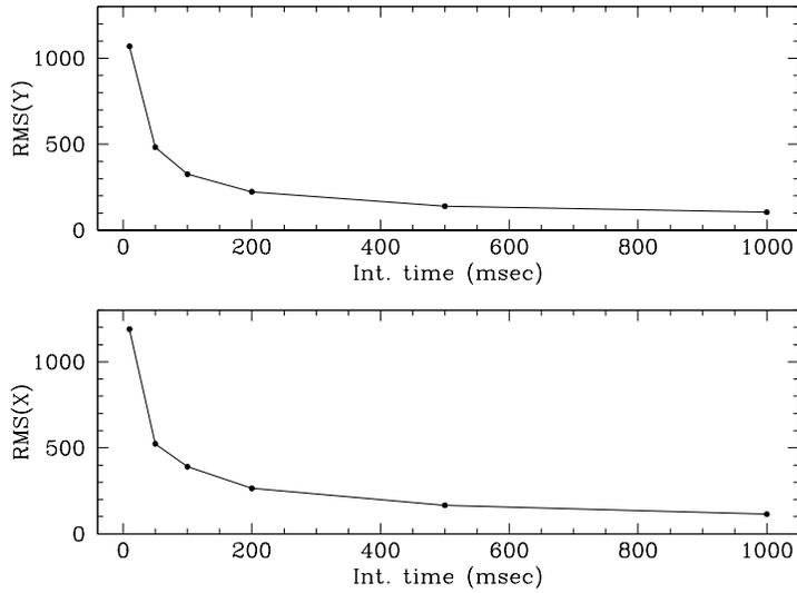
Figure 14: The RMS value on the guide signal for different integration times.
