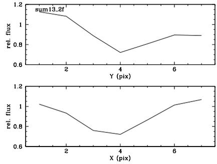
Figure 7: The relative flux as a function of x and y position in the central row and column of the previous summed image. The raster step size is  $250\mu\text{m}$  ( $0.13\text{arcsec}$ ) and the feedfiber is  $105\mu\text{m}$  or  $0.23\text{arcsec}$  in the sky.
