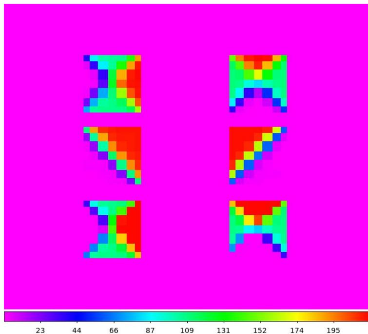
Figure 11: The guide signal as a function of raster position for the small feed fiber with the 0.23arcsec spot size. The raster had steps of  $250\mu\text{m}$ .
