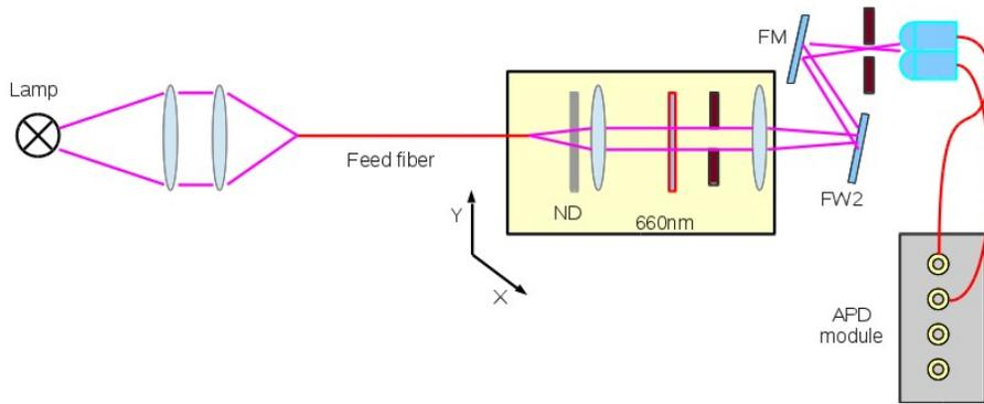
Figure 1: The test setup. The halogen lamp provides the light to the feed fiber. The end of the feed fiber is reimaged through a factor four beam expander, delivering an f/45 beam on the lenslets. The location of the ND filters and interference filters are shown. The mirrors in the filter wheel (FW2) and fold mirror (FM) are red pass mirrors suppressing the light blueward of 600nm. The fiber bundle from the lenslets to the APD module is also indicated.
