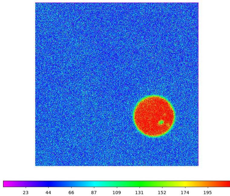
Figure 8: The pinhole image on the Apogee camera. The smooth illumination is obvious as is the sharp edges of the spot.
