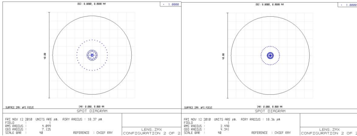
Figure 9. Spot patterns on the natural star focal plane. Left: when all optics are in their nominal position as indicated in Figure 7. Right: when a 50µm shift on M2 has been applied to compensate for a 10mm differential movement between the ARGOS WFS and the Calibration Unit.
