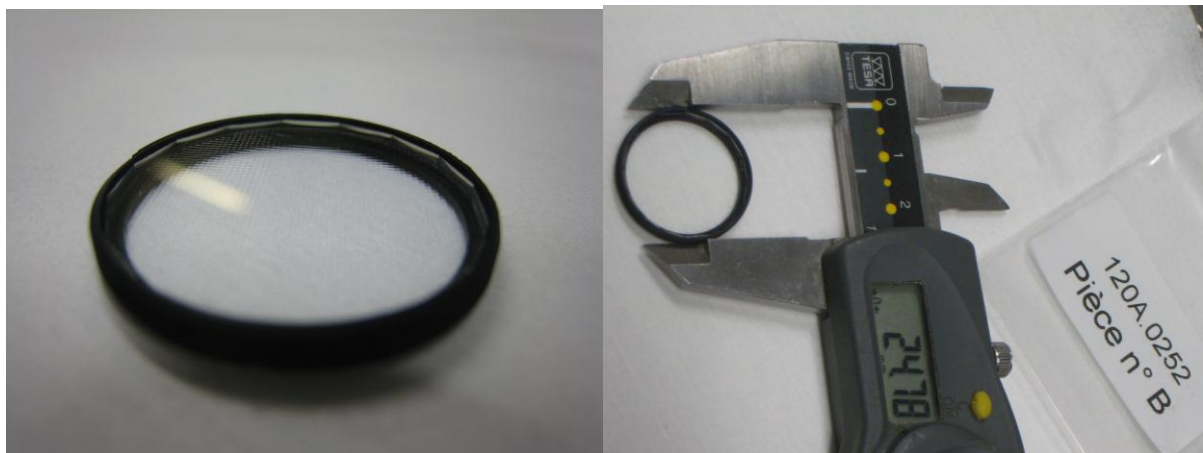
Figure 1. Left: picture of one unit of ARGOS lenslet array. Right: measurement of the external diameter of the pieces. 25mm is the upper limit to fit into the mechanical mount.
